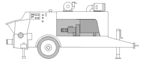
Figure 1: Detail of typical grout pump
