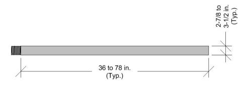
Figure 2: Detail of typical grout casing
