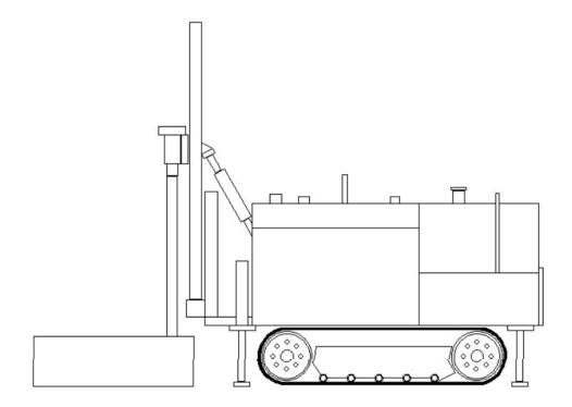
Figure 3: Detail of typical rotary wash drilling rig
